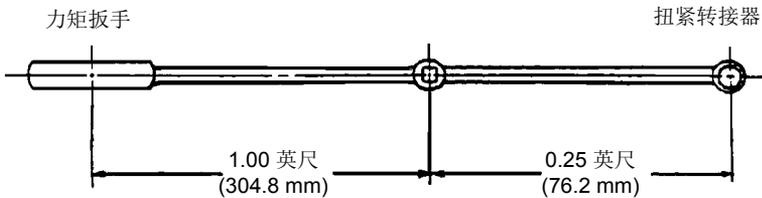
$$\frac{(\text{所需实际力矩}) \times (\text{力矩扳手长度})}{(\text{力矩扳手长度}) + (\text{转接器长度})} = \text{力矩扳手读数}$$
